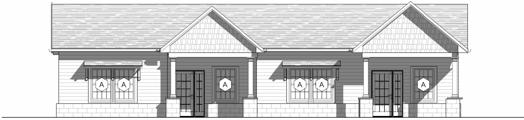
1 BUILDING TYPE A - FRONT ELEVATION 1/8" = 1'-0"
