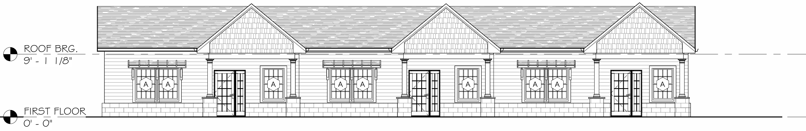
5 BUILDING TYPE B - FRONT ELEVATION 1/8" = 1'-0"
