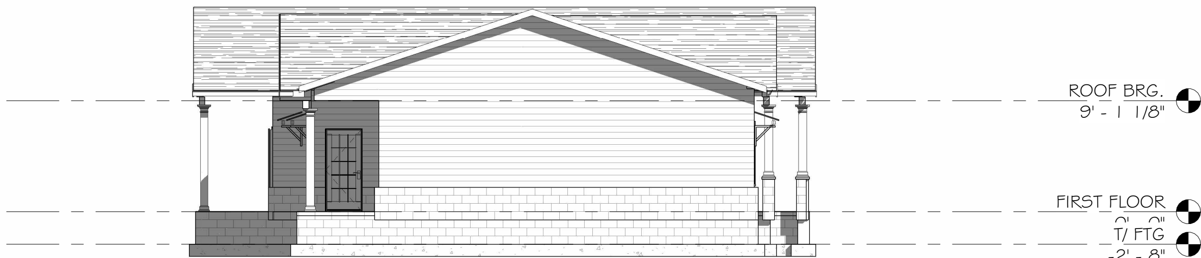
3 BUILDING TYPE A - SIDE ELEVATION 1 1/8" = 1'-0"
