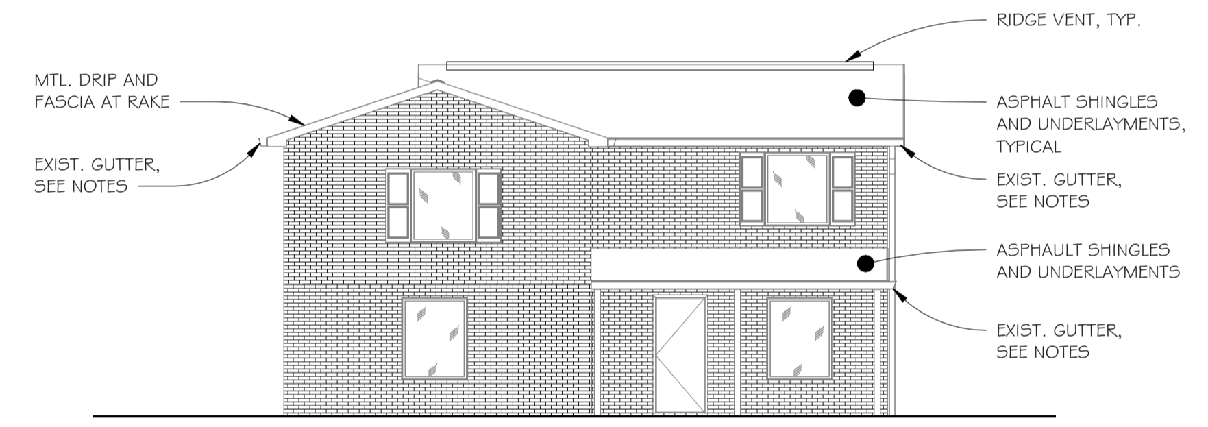
2 BUILDING TYPE D ELEVATION 1/8" = 1'-0"
